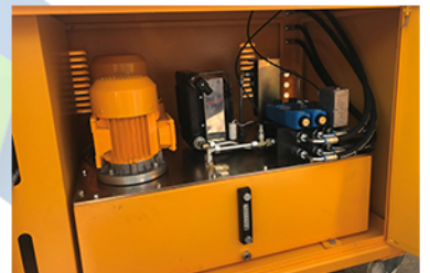
power pack unit for material testing machine
